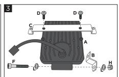
Tighten the top bracket (C) to the Acerbis headlight (A) using the screws (D). Assembly the lower bracket (B) through the screw (F), the washers (L) and then nut (H), without tightening.
