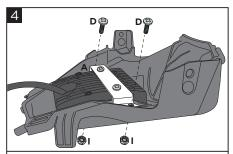
Insert the headlight (A) and secure at the frame with the remaining bracket screws (D) and the nuts (I).
