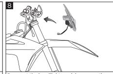
Remount the headlight mask by connecting the connector.
