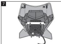
Fix the internal frame in the mask using the original screws (M).
