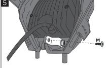
Slightly tighten the lower bracket screw (F) previously entered, putting in position the hole for the upper screw (M). Assemble the screw (M) and tighten both screws fully.
